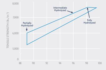
Tensiles determined on Instron Tester: 1.7 mil dry film thickness equilibrated to 73°F at 50% RH
