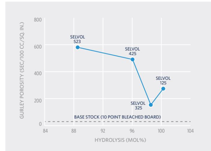
FIGURE 7: Surface Effects vs. Degree of Hydrolysis
