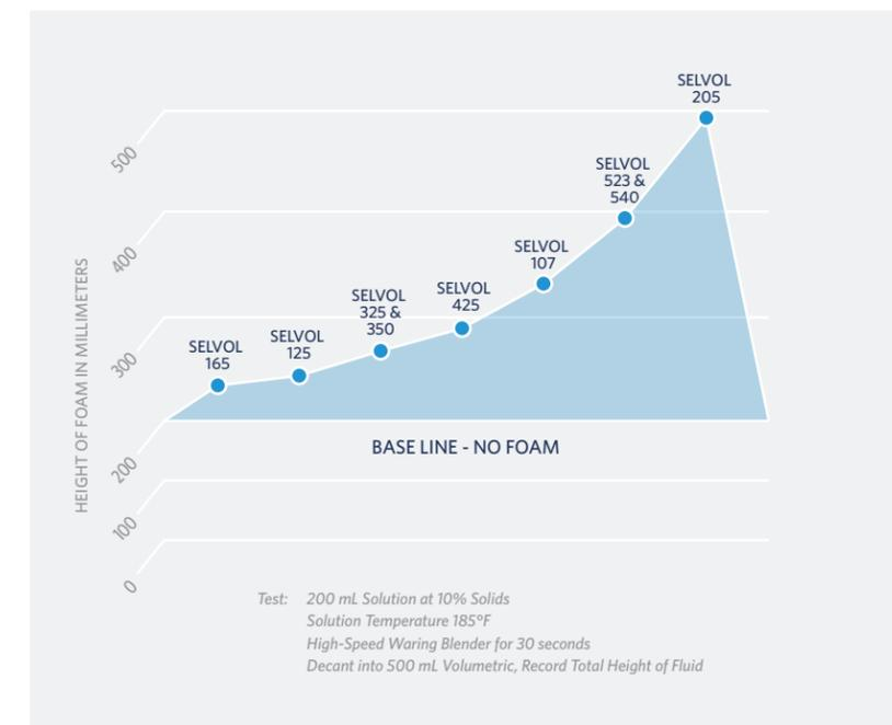
FIGURE 4: Foaming Characteristics of Selvol Polyvinyl Alcohol
