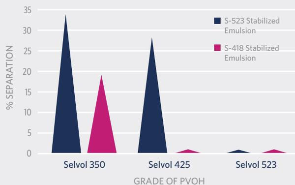
\* Compatibility test run by mixing 50/50 by volume emulsion and 10 wt % PVOH solution. The mixture was then diluted to a viscosity of 1000 cPs and stored for 1 week at 70 °C.
