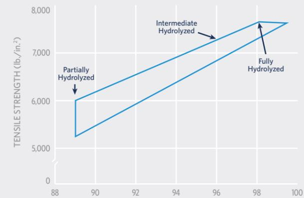
\*Tensiles determined on Instron Tester: 1.7 mil dry film thickness equilibrated to 73°F at 50% RH
