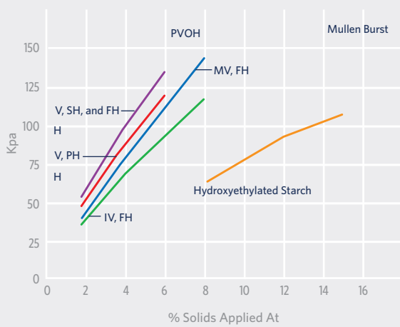
FIGURE 1: Laboratory Size Press Study Polyvinyl Alcohol vs. Starch on 77 g/m 2 Base Paper
