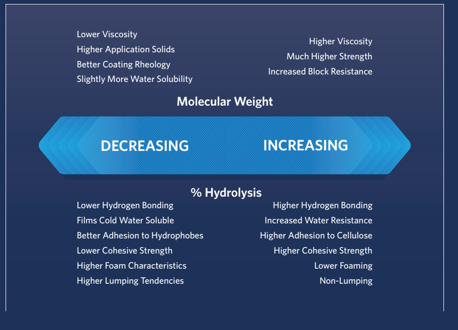
FIGURE 3: Changes in PVOH Properties in relation to Molecular Weight and Hydrolysis Level
