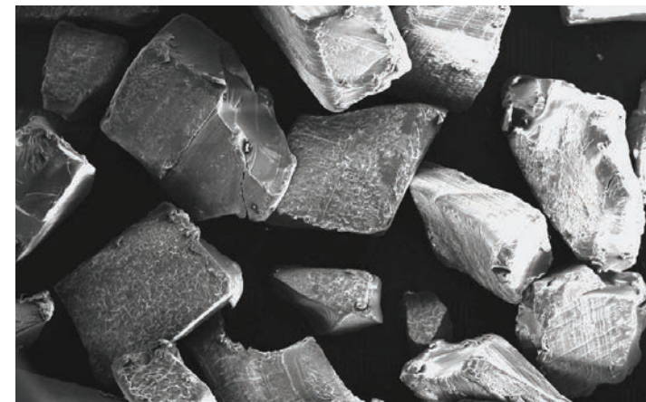
Top: Selvol PVOH Granules; Bottom: Selvol under a scanning electron microscope.
